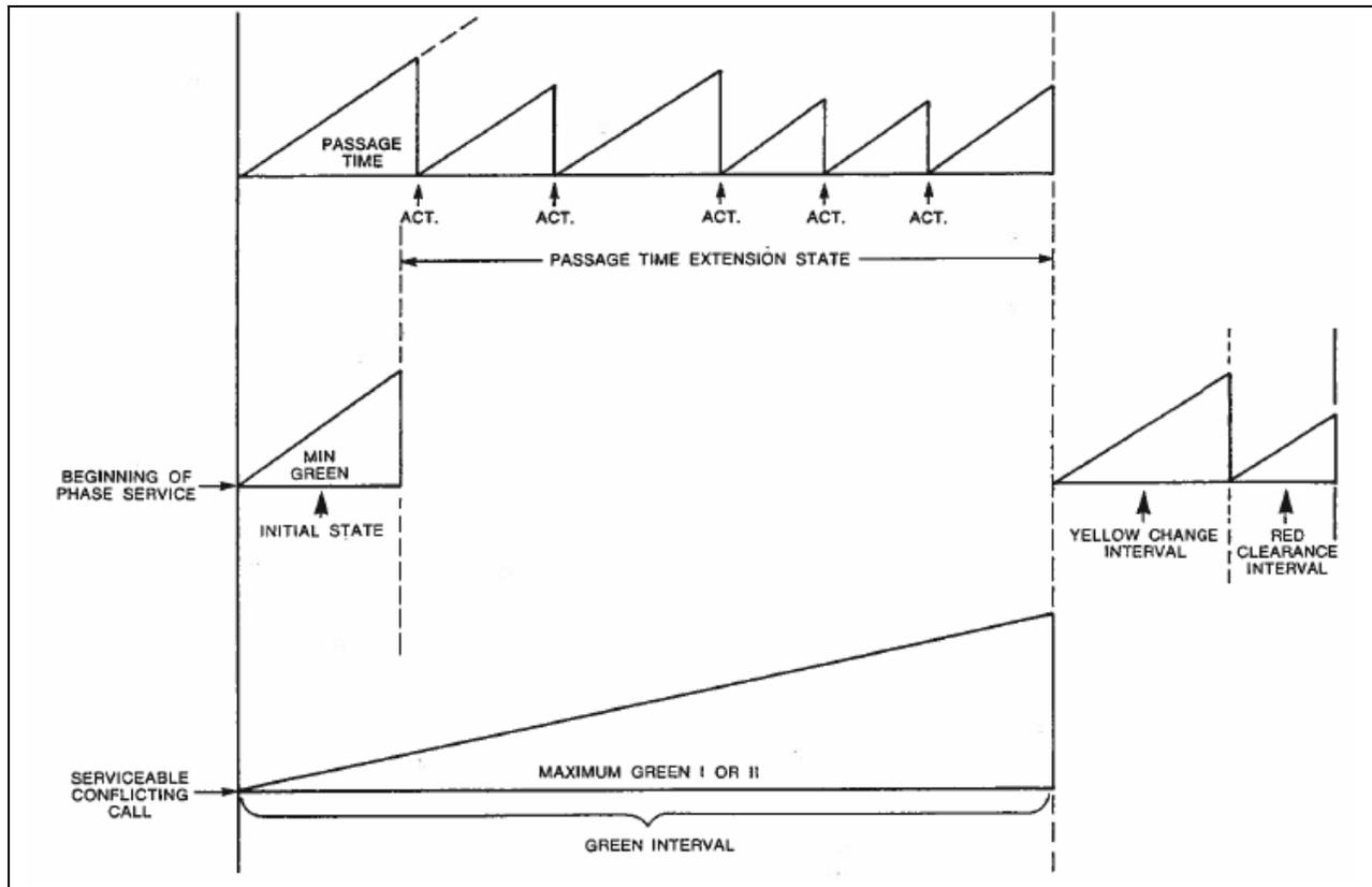
**Figure 2-4 Typical Standard Timing Diagram**
