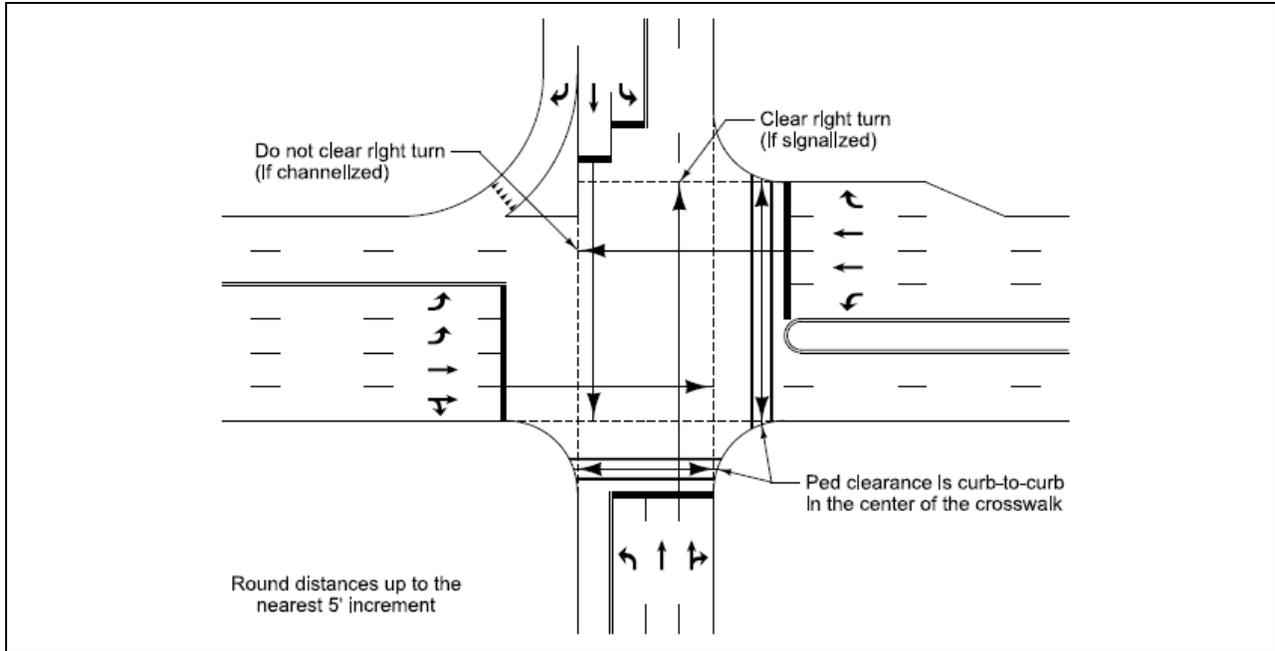
**Figure 2-8 Through Movement Clearance Distances**
