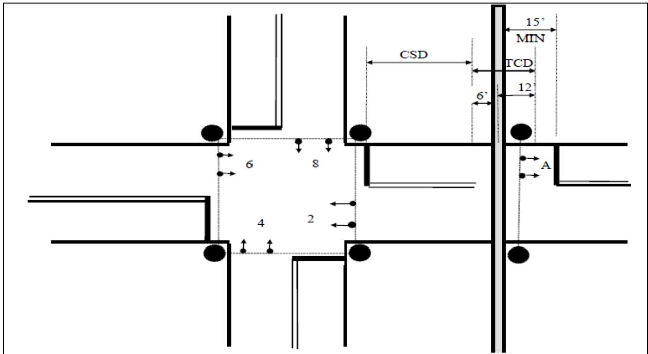
**Figure 5-2 TCD and CSD Measurement Guide**
