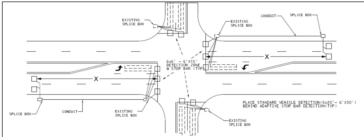
**Figure 4-3 Inductive Loops for Traffic Adaptive**
