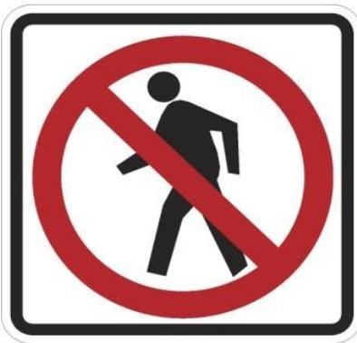
Intersections that present a serious and consistent safety concern for pedestrians should prohibit crossings using sign R9-3-12 (No Pedestrian Crossing). Also, signal phasing may require pedestrians to only cross along a single approach. Restricting pedestrians at an intersection can be accomplished through appropriate signing that provides guidance to preferred crossing locations.
