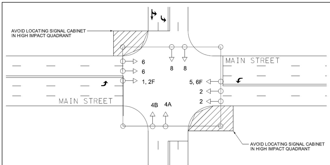
**Figure 4-2 High Impact Signal Cabinet Locations**
