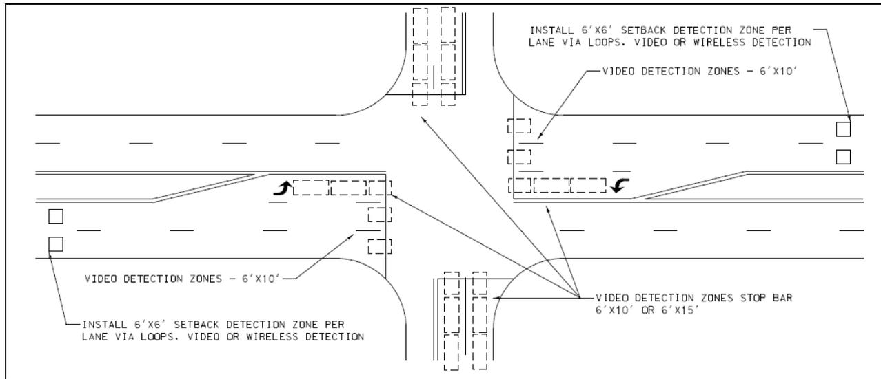
**Figure 4-6 Video Detection Zones for Traffic Adaptive**
