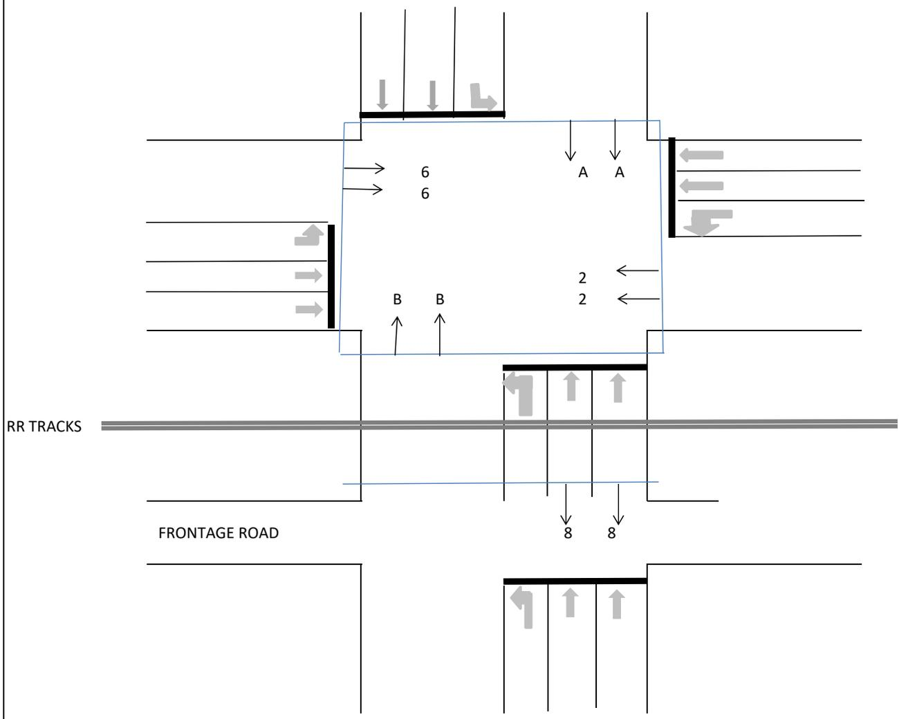
A TIMED OVERLAP WILL EXTEND THE GREEN TIME FOR OVERLAP SIGNAL HEADS (A AND B AS SHOWN IN THIS EXAMPLE) FOR THE TIME SPECIFIED IN THE CHART. TIMED OVERLAPS ARE COMMONLY USED TO PREVENT VEHICLES FROM GETTING CAUGHT IN THE SHORT STORAGE AREA BETWEEN THE FRONTAGE ROAD AND INTERSECTION. NOTE THAT BOTH APPROACHES UTILIZE TIMED OVERLAPS TO ENSURE HEADS A AND B GO TO YELLOW AND RED SIMULTANEOUSLY.
