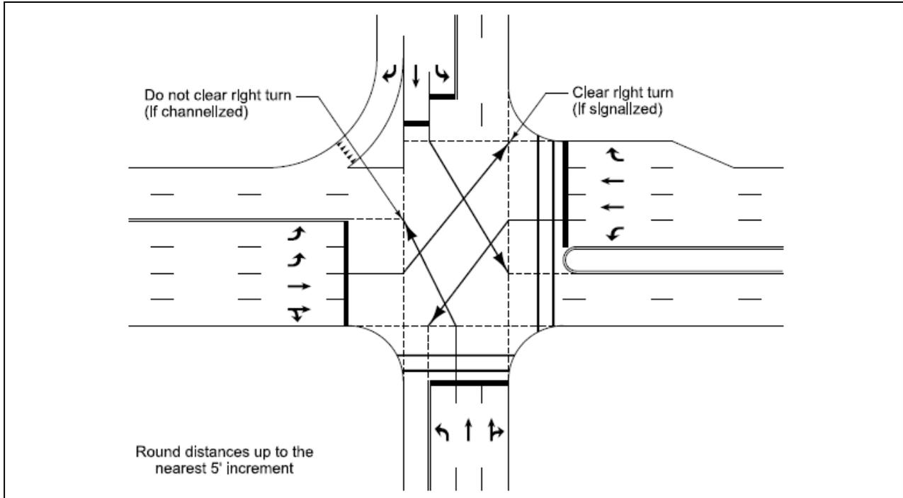
**Figure 2-9 Left Turn Movement Clearance Distances**
