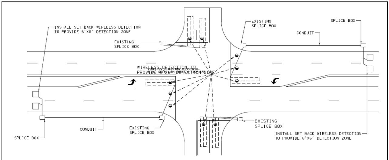
**Figure 4-5 Wireless Detection with Inductive Loops for Traffic Adaptive**
