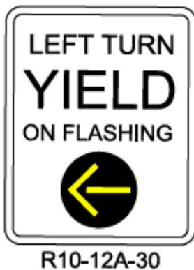
SCDOT sign R10-12A-30 explains the flashing yellow arrow operation to approaching motorists and should be placed adjacent to the FYA signal head.
