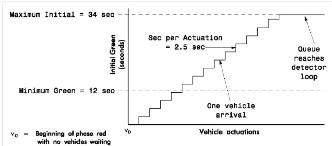
**Figure 2-2 Added Initial Time Example**
