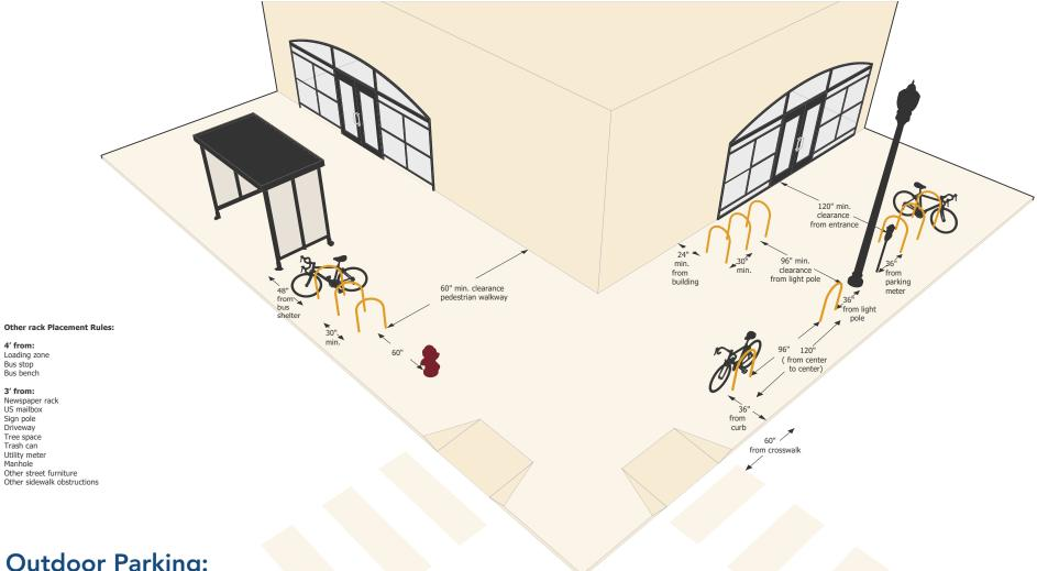
Figure 4: Outdoor bike parking spacing and dimensions
