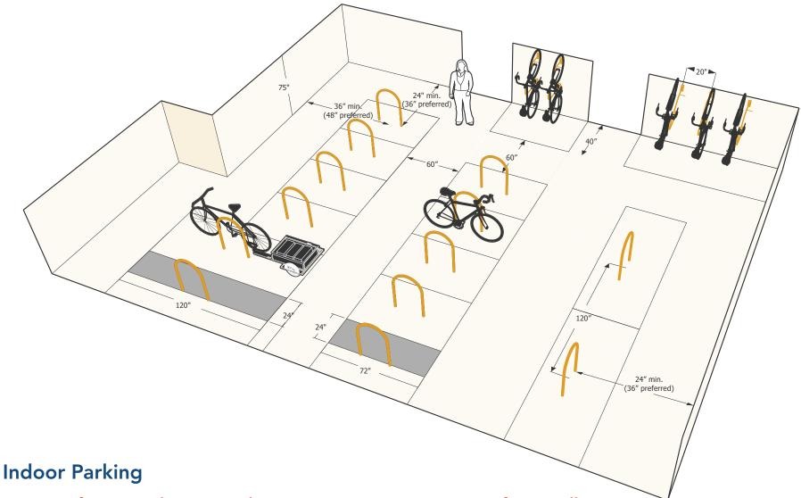
Figure 3: Bike Room Rack Dimension/Spacing
