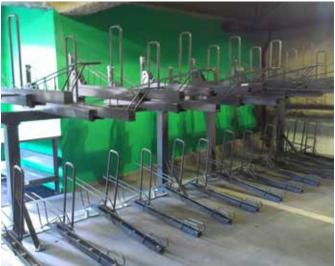
Indoor bike parking can include vertical or double-tier racks, as long as the racks are securely bolted to the building and it is possible to lock the bike frame and one wheel with a standard U-lock.
